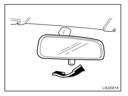
The day/night adjustment allows you to adjust the mirror to avoid glare from any headlamps behind you. Push or pull the tab for daytime/night use.
